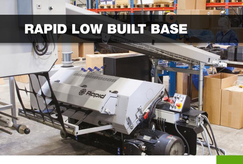
The new Rapid 300-Series LBB, Low Built Base, granulator is an extremely low built granulator series available in three widths, up to 1500 mm.
