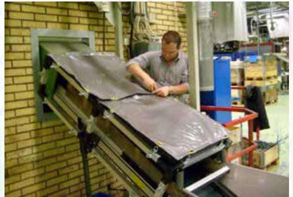
The main areas for Rapid MSS is as sound enclosure for granulators and their transport system.
