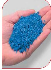
**Highest-quality regrind** The Rapid cutting technique, comprising clean double scissors-cutting action and constant cutting circle, produces granules of a uniform size with minimal dust content even with the toughest materials.
